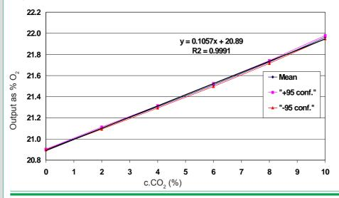
Carbon dioxide increases the diffusion rate of oxygen, increasing the apparent oxygen concentration.
