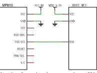
The simplest circuit connection of UART
