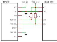
Electrical connection of IIC interface
